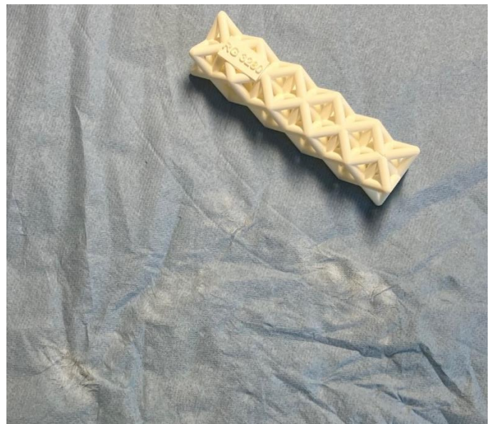
Chalkiness after thermal-treatment
